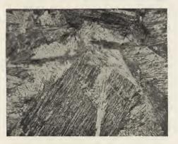
Fig. 28. (x 35 Diameters. Vertical Illumination.) Same as Fig. 27 after quenching.
